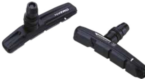
877.12 Pattino V-BRAKE High Range asimmetrico Portapattino in alluminio Lenght 72 mm Degree 0°
